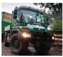
AC Price built the sub-frame, chipbox and three-point linkage at its factory in Ingleton, adding hydraulics and a rear PTO, so that the chipper can be operated from the back of the vehicle, as well as the front.
